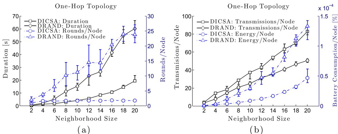
**Fig. 4.** Evaluating the execution performance of DICSA and DRAND in various-size one-hop networks. (a) Execution duration and average number of rounds per node. (b) Average number of packet transmissions per node and average battery consumption per node. Since DICSA does not impose any distance between the nodes reserving slot, it provides shorter algorithm execution duration and lower energy consumption.
