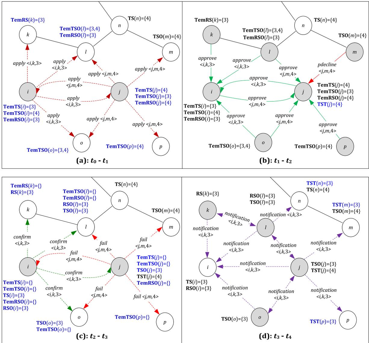
**Fig. 3.** A sample slot reservation scenario. Gray circles show the transmitting nodes during each interval. Solid arrows and dotted arrows represent unicast and broadcast transmissions, respectively.
