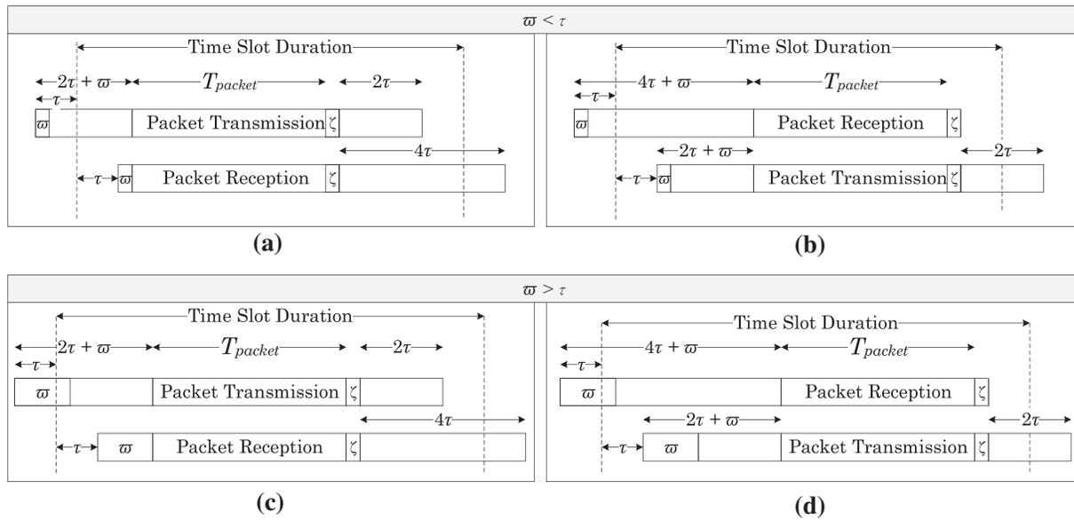
**Fig. 8.** Minimum time slot duration with respect to time synchronization accuracy ( $\tau$ ) and radio switching delay ( $\omega$ ). (a) and (b)  $\omega < \tau$ . (c) and (d)  $\omega > \tau$ . Irrespective to the relationship between  $\tau$  and  $\omega$ , the minimum time slot duration should be  $4\tau + \omega + T_{packet} + \zeta$ . In this paper we assume  $\tau = 1$  ms,  $\omega + \zeta = 1$  ms, and  $T_{packet} = 18.33$  ms.
