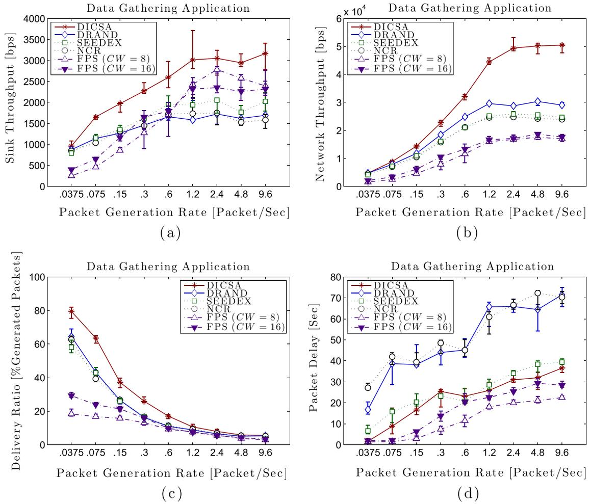
**Fig. 9.** Performance evaluation of various scheduling algorithms versus traffic rate in data gathering applications. Compared with DICSA, the lower throughput and delivery ratio of DRAND and NCR is due to the lower spatial reuse of node scheduling which results in buffer overflow and packet loss. Packet losses caused by collisions reduce the throughput and delivery ratio of SEEDEX and FPS, compared with DICSA.
